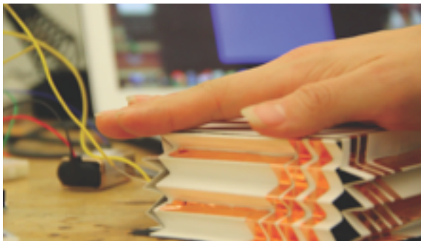
Figure 16: 3D Physical Structure Composed of Compositing Sensors & 2D Digital Representation
