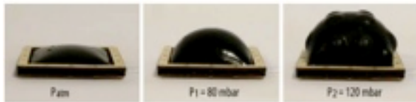
Figure 3: As the air pressure increases the surfaces deform.
